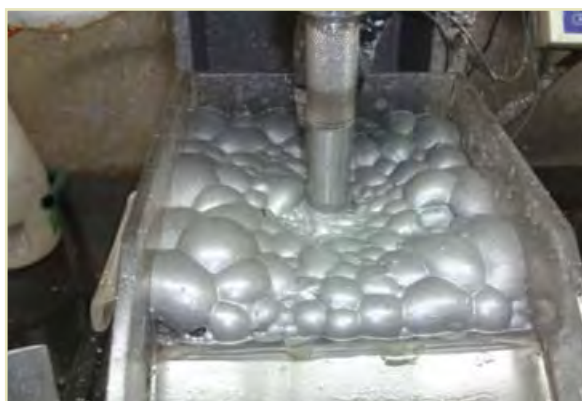
Figure 10: Flotation test of Romang Island polymetallic sulphide composite sample
