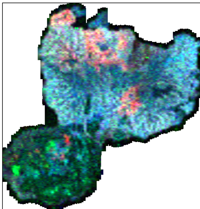
Figure 3 Radiometry ternary image plot (Red: Potassium, Green: Thorium, Blue: Uranium)
