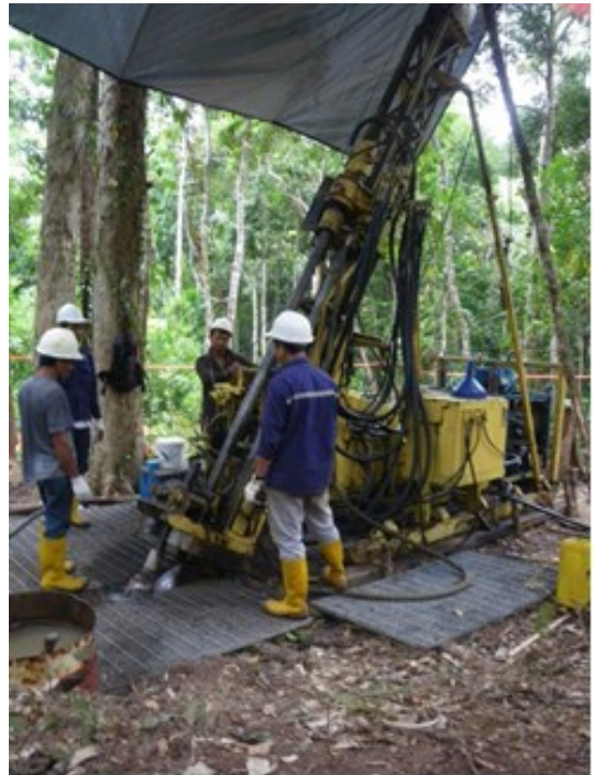
Figure 14: Robust diamond rig (drilling LWD367)
