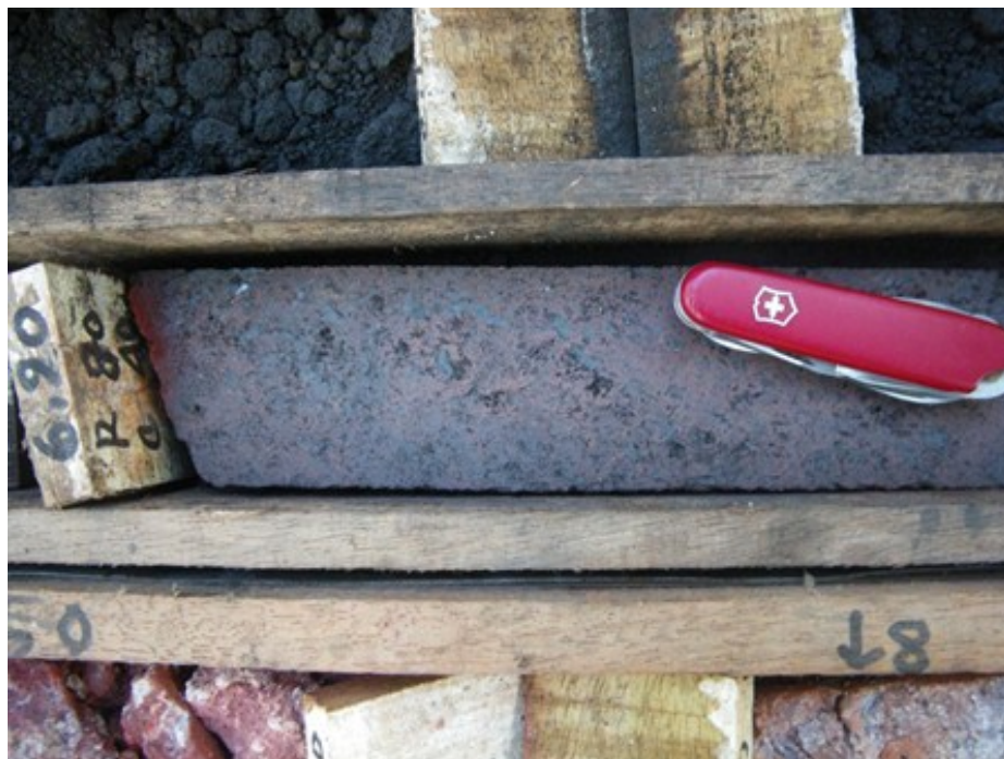
Figure 17: Inspection of LWD 262 at 6.2m down hole where >3m @ 41.5% Mn was reported
