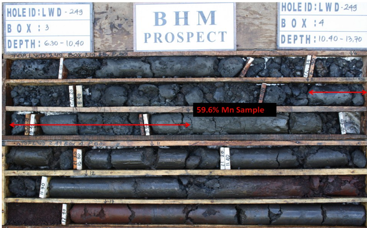
Figure 5: Core Tray containing high grade manganese mineralisation (ASX release 12/12/12)
